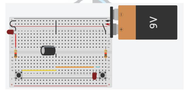
**Working:** This circuit demonstrates the behavior of a capacitor with separate charging and discharging controls, and provides visual feedback through two LEDs.
